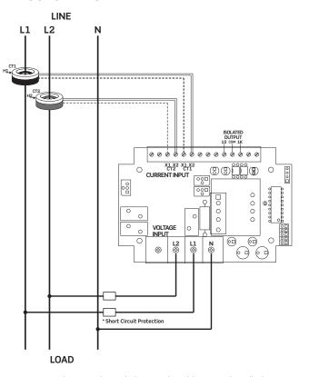
Leviton recommends solid core transformers (CTs) for revenue-grade accuracy. Our 100A and 200A color coded CTs assist with correct installation by indicating phase monitored. Split core CTs are also available upon request for applications where power cannot be interrupted during installation. Our 100-800 Amp Split Core CTs offer +/-1.0% accuracy.
