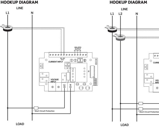
Leviton recommends solid core transformers (CTs) for revenue-grade accuracy. Our 100A and 200A color coded CTs assist with correct installation by indicating phase monitored. Split core CTs are also available upon request for applications where power cannot be interrupted during installation. Our 100-800 Amp Split Core CTs offer +/-1.0% accuracy.
