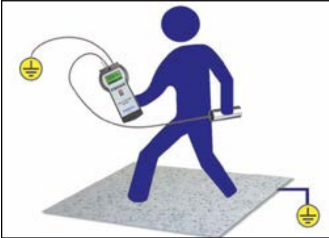
Figure 3. Setup of the Body Voltage Meter
