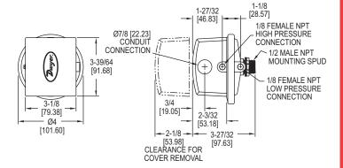
Essential for industrial environments, the Series 1800 Low Differential Pressure Switch for General Industrial Service combines small size and low price with 2% repeatability for enough accuracy for all but the most demanding applications. Set point adjustment inside the mounting stud permits mounting switch on one side of a wall or panel with adjustment easily accessible on the opposite side. UL and CSA listed, and FM approved. For use with air or compatible gages.
