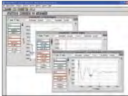
By double-clicking on an event, the software displays all trends and waveforms related to this event.
