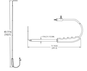
The Model 166T Telescoping Pitot Tube is a convenient adjustable length instrument for sensing air flow in a wide range of duct sizes, extending your reach to 36 inches (91 cm). It is ideal for almost any air velocity measurement where permanent mounting is not required. Because of the very small sensing holes on the tip, flow must be reasonably clean and free from particulates which could cause blockage.
