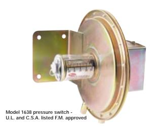
**Our highest precision** conventional large diaphragm pressure switch provides maximum dependability. In addition it incorporates a visible set point indicator for maximum convenience. U.L. and C.S.A. listed, F.M. approved for general service, these switches are suitable for most applications in air conditioning and industrial service. Electrical capability of 15 amps handles most small electrical loads.
