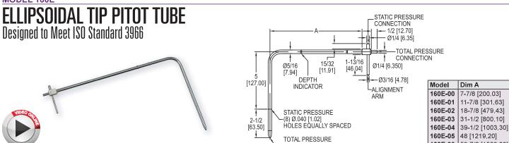
The **Series 160E Ellipsoidal Tip Pitot Tube** uses a precision crafted tip configuration, which allows air to pass smoothly with minimum turbulence for consistent, reliable readings. Sliding depth indicators grip firmly to ensure uniform insertion when measuring traverses across ducts. Total and static pressure taps are  $1/4^{\prime\prime}$  (6 mm) and are permanently silver soldered to the connection block, making them leak-proof and durable.
