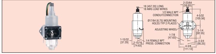
**Same rugged construction** as used in Series 1000W plus explosion-proof design are combined in this new unit. UL listed for Class I, Groups A, B, C & D; Class II, Groups E, F & G. Bellville spring movement permits mounting of control in any position and helps prevent contact chatter. High over-pressure protection and vibration resistance are also featured.
