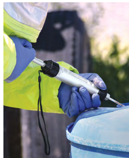
First responder uses RAE Systems colorimetric tubes and hand pump to measure VOC levels inside a barrel.
