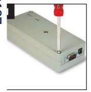
eparate the two halves of e gauge housing by loosling the captive screws. len pull the two halves part.
