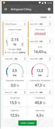
Added refrigerant is displayed in g/kg increments on the manifold/app.
