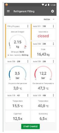
Added refrigerant is displayed in g/kg increments on the manifold/app.
