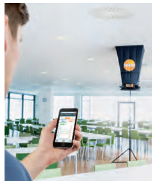
Bluetooth App allows for hands free operation, displaying measurement data on mobile devices and finalizing and sending the measurement report via email from the job site
