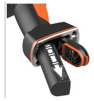
Push the new battery all the way into the rechargeable battery slot until it is flush with the bottom of the handle.
