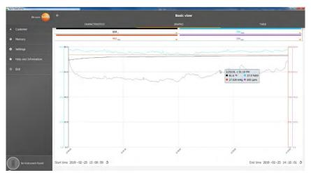
Clicking on one of the four channels opens the selection of measurement parameters recorded during the measurement. The measuring parameters can easily be assigned to the individual channels via the probe ID and measuring unit or selected as **not assigned**.
