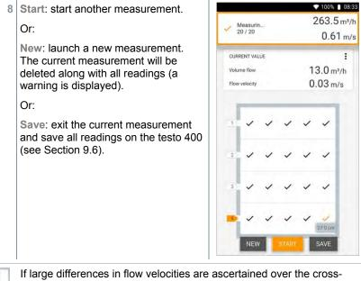
If large differences in flow velocities are ascertained over the crosssection, the number of measuring points must be increased. The number of measuring points is then adequate if the measurement value for each area is representative for its immediate surroundings, i.e. if it can be regarded as a genuine mean value for its portion of the area.
