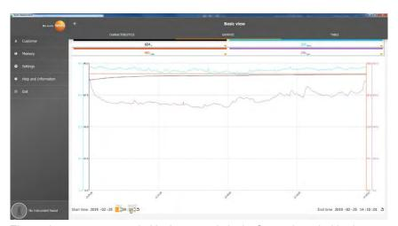
The total measurement period in the example in the figure above is 60 minutes. After changing the start time, only the last 10 minutes of the measurement are displayed in the graphic in accordance with the selection. Adjusting the time enables the measuring values to be analyzed in detail. To display the complete measurement period in the graphic once again, click on
