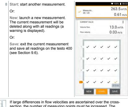
section, the number of measuring points must be increased. The number of measuring points is then adequate if the measurement value for each area is representative for its immediate surroundings, i.e. if it can be regarded as a genuine mean value for its portion of the area.
