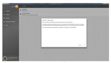
As soon as the testo 400 is connected via a USB cable to a computer, **Connected to testo 400 – Synchronizing** is displayed at bottom left. A message about data transfer is displayed. Confirm by pressing OK to transfer all customer and measurement data from the testo 400 to the software. The testo 400 memory is then empty. Depending on requirements, customer and measurement data as well as measuring site information can be transmitted back.
