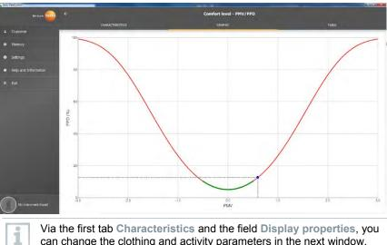
can change the clothing and activity parameters in the next window. This recalculates the PMV/PPD values and also the graphic. In order to be able to compare different calculations/graphics with each other, you need to save the respective CSV and PDF files. The calculations are overwritten in each case - it is therefore not possible to view different results of a measurement at the same time.
