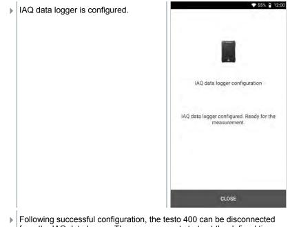
Following successful configuration, the testo 400 can be disconnected from the IAQ data logger. The measurement starts at the defined time or as soon as the setup has been completed (if the start time has been set to manual). The green LED on the IAQ data logger flashes rapidly at short intervals.
