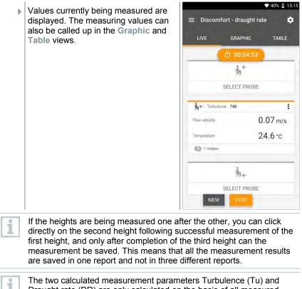
Draught rate (DR) are only calculated on the basis of all measured values. This means that these two values are displayed at the end of the measurement and are not calculated for each time point of the measurement.
