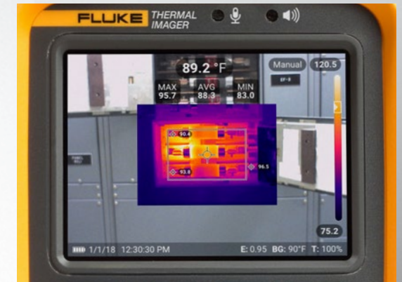
Improved interface helps to quickly identify min/max temperatures.
