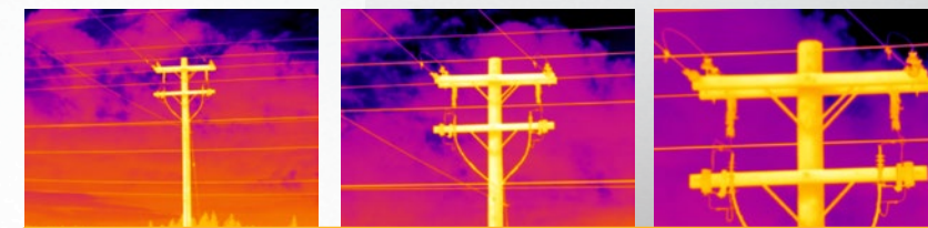
Standard (left), 2x telephoto (center) and 4x telephoto (right)—see the right level of critical infrared detail
