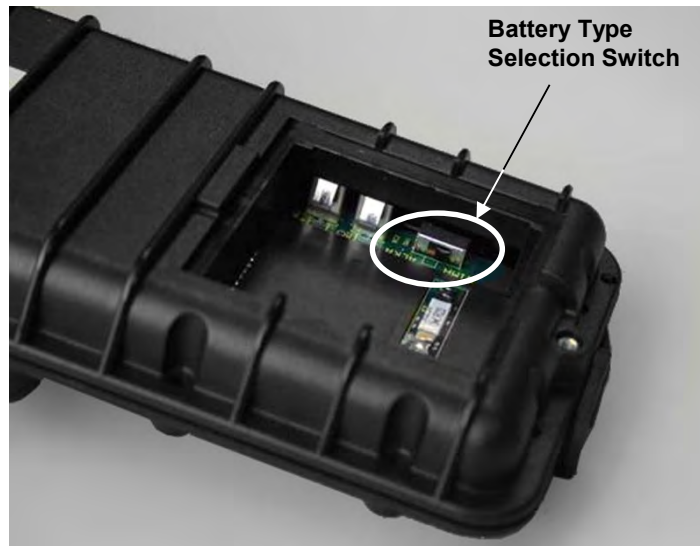
Figure 2-1 Location of Battery-Type Selection Switch
