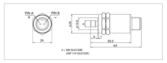
The vibration transducer SLD122B and SLD122F are piezoelectric accelerometers of compression type with built-in preamplifier, designed for vibration monitoring of industrial machinery. The electrical signal is isolated from the transducer housing.
