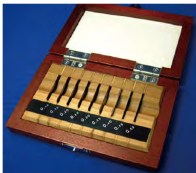
Figure 33 Ultra-thin gauge block set
