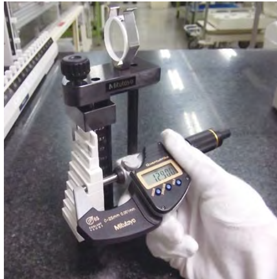
Figure 47 Micrometer-check gauge block holder (developed in 2002)
