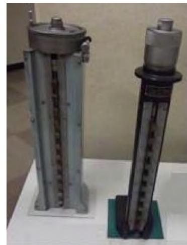
Figure 21 Original Height Master (height check micrometer)
