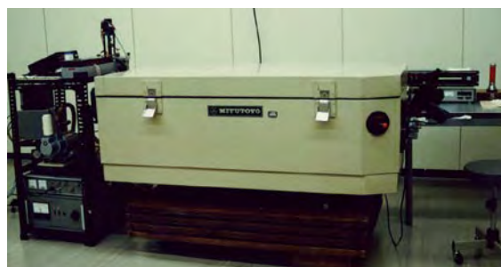
Figure 35 Interferometer for measuring long gauge blocks
