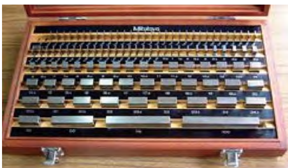
Figure 30 103-piece gauge block set (manufactured by Mitutoyo)
