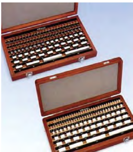
Figure 36 Mitutoyo steel gauge blocks (back) and ceramic gauge blocks (front)
