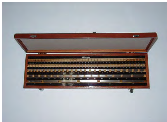
Figure 48 122-piece gauge block set (developed in 1999)
